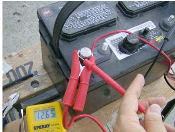
Checking the voltage
